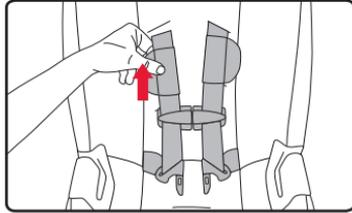
6. From the back of the infant car seat, slide the harness straps completely onto the harness yoke. Ensure that the adjuster strap is not twisted.
