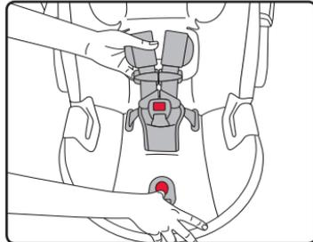
2. Locate the harness yoke on the back of the infant car seat and slide one harness strap off of the yoke.
