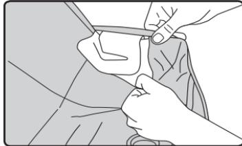
7. Pull cover from around harness adjust button and lift the seat cover away from the seat shell.
