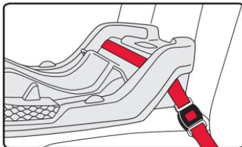
3. Press the base firmly into the vehicle seat while removing all slack from the vehicle seat belt.
