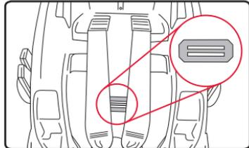
3. Turn the buckle strap retainer so that the short side will go through the slot in the infant car seat shell and cover.
