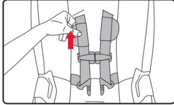
2. Loosen the harness by pressing down the harness adjuster button while pulling both harness straps forward.
