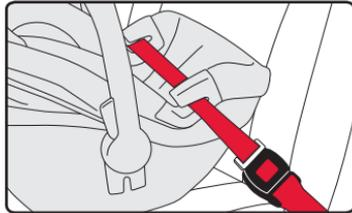
5. Push the infant car seat firmly into the vehicle seat while removing all slack from the vehicle belt.
