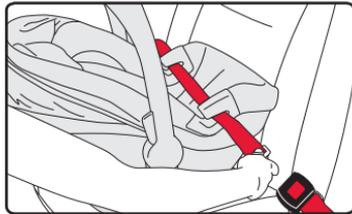
4. Verify that the vehicle belt is not twisted and then buckle. Lock your vehicle seat belt system as instructed by your vehicle owner's manual.
