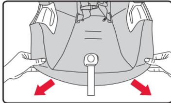
8. Slide each side of the harness, with the buckle tongue and chest clip, through the cover and pull the cover off of the shell.
