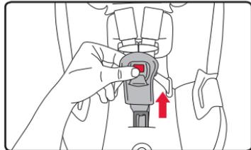
5. Push the retainer through the slot in the cover and shell for the appropriate buckle position.
