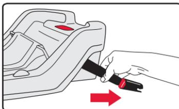
3. Place the base on the vehicle seat and press the lower connectors onto their adjacent vehicle lower anchors until a click is heard.
