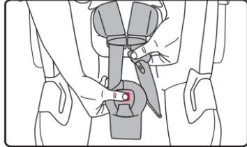
2. Locate the buckle strap retainer on the bottom of the infant car seat and pull away from the seat to loosen.
