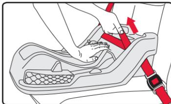
4. Hold the vehicle shoulder belt tightly and slide firmly under the lock-off on the side of the base opposite the buckle.
