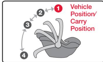
To adjust, press and hold both handle release levers and rotate the handle to the chosen position.
