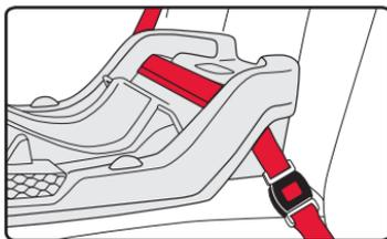
3. Press the base firmly into the vehicle seat while removing all slack first from the lap portion and then from the shoulder portion of the vehicle seat belt.
