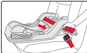
2. Ensure that the vehicle seat belt is not twisted and buckle.
