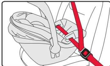
5. Push the infant car seat firmly into the vehicle seat while removing all slack from the lap portion and then the shoulder portion of the vehicle belt.
