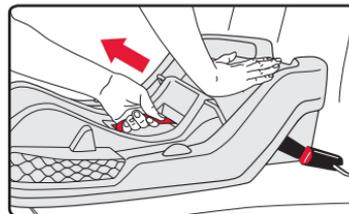
5. Feed excess webbing back into base and ensure that lower connector straps are flush with the base.
