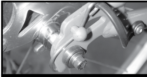
FIG. 6 - Fork Hook Correctly Installed
