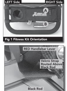
Fig 2 Velcro Strap Routing
