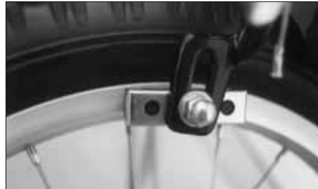
Fig. 6a - Brake pads shown aligned to rim. Patins de freins alignement correct. Bremsklötze in korrekter Stellung zur Felge.
