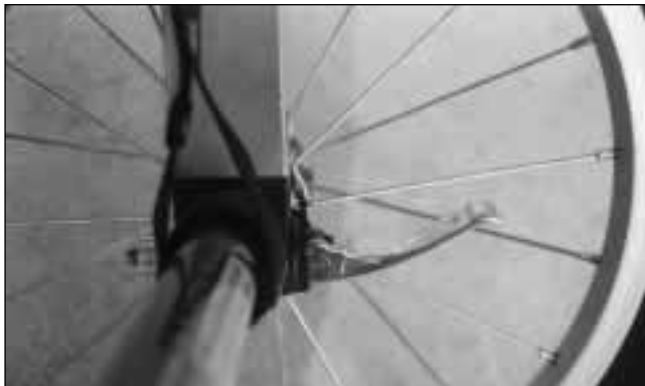
Fig. 4 - A.F.O.D. (Anti Fly Out Device) correctly attached. Sangle anti projection correctement attachée. Federwegbegrenzung (Anti-Fly-Out-Device) in korrekter Befestigung.
