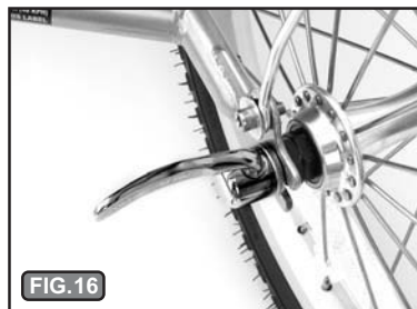
FIG. 16 QR lever perpendicular to dropout face.
