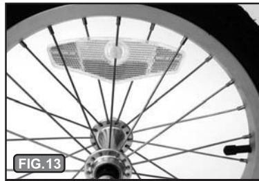
FIG. 13 Wheel reflector correctly positioned.
