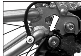
FIG. 2 Trailer in extreme counter-clockwise rotation showing contact between derailleur pivot housing and trailer fork. AVOID this condition. If you believe this has occurred, inspect your derailleur, QR, and pins for damage.
